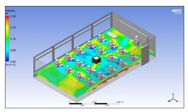
The collection point at floor level and the returned clean air at the top of the unit address the descending flow of droplets and ensure a circular flow throughout the room.
