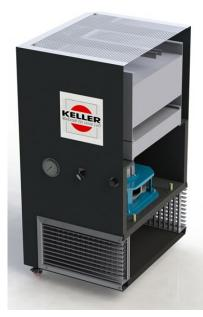
The two hanging HEPA filter stages remove 99.995 percent of all particulate from the air, even tiny particles measuring between 0.1 and 0.3 micrometers. The first filter exchange can be expected after 2 to 5 years, depending on the intensity of use. A sensor indicates the proper time for a filter change.
