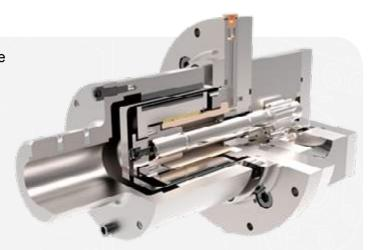
The magnetic coupling lends itself to conveying poisonous or flammable substances, as well as for operation at high system pressures. Special versions can be used for inlet pressures of up to 500 bar (7.252 psig).
