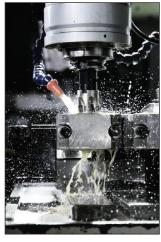
Water-soluble aerosols are released from coolants during cutting processes.
