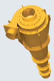
Left: Cavex<sup>®</sup> hydrocyclones feature a unique laminar spiral inlet geometry designed to deliver excellent efficiency and capacity, and longer wear life than conventional involute or tangential fed cyclone designs.
