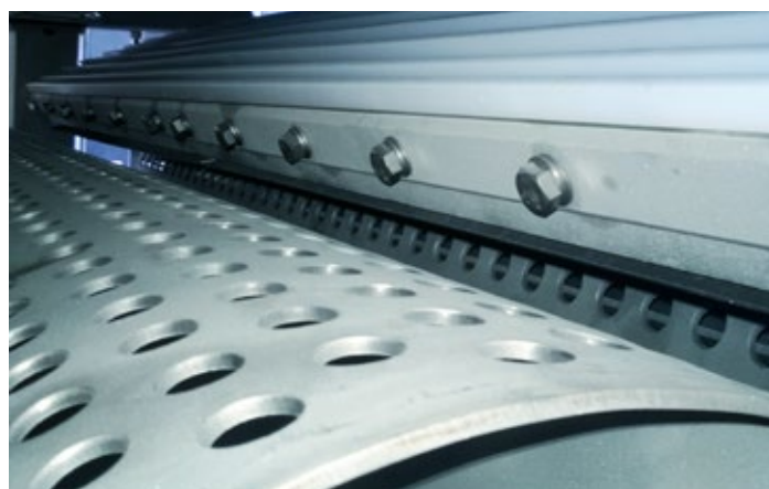
7, 8 or 12 rolls for lowest residual moisture of final product
