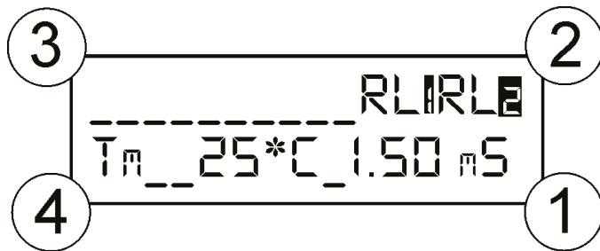
**Area 1** = Display of chemical conductivity measurement
